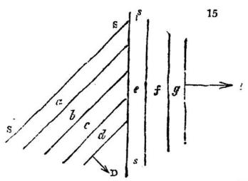
the series of strata marked a b c d are parallel in one set, and e f g in another; but their directions, or strikes, (S, S and s s) on the surface differ, and the lowest of the upper set (e) rests in one place on a, in another on b, in another on c or d.; the dips, D and d, are in different directions.
