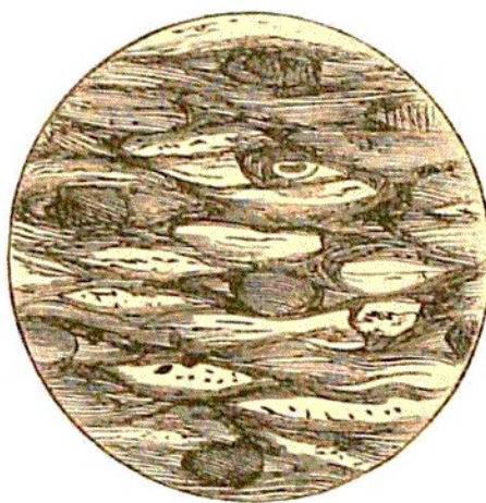
FIG. 22.—Sheared Red Sandstone forming now a Micaceous Schist, Keeshorn, Ross-shire. The pebbles are crushed and elongated, and the feldspar materials have been partly converted into mica.
