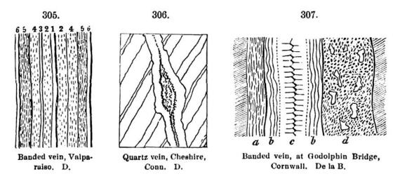
But granitic veins are sometimes banded, as in Fig. 305, in which 1, 3, and 6 are bands of quartz; 2 and 4, bands having the structure of gneissoid granite, and 5 that of gneiss. Fig. 306 contains a two-banded vein of quartz. It illustrates the usual mode of origin of bands, showing that they are layers made by deposition against the two walls. It is also a vein of copper ore, the ore lying in the wider open portions of the vein.
