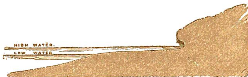
Fig. 161.—Section of a Beach defined by High- and Low-water Mark.
