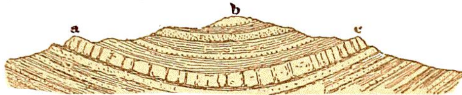
Fig. 245.—Trough, or Syncline, with strata ( a c ) rising from each side of a central axis ( b ).
