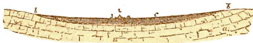
Fig. 106.—Diagram illustrative of the theory of Artesian Wells.
