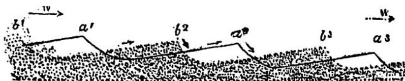
Fig. 91.—Diagram of Ripples in blown Sand. The ridges b^1 , b^2 , b^3 , impelled in the direction of W W, successively come to occupy the hollows a^1 , a^2 , a^3 (B.).
