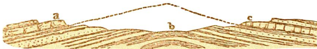
Fig. 244.—Arch, or Anticline, which has been denuded by the removal of beds, as shown by the dotted line a c above the axis b .
