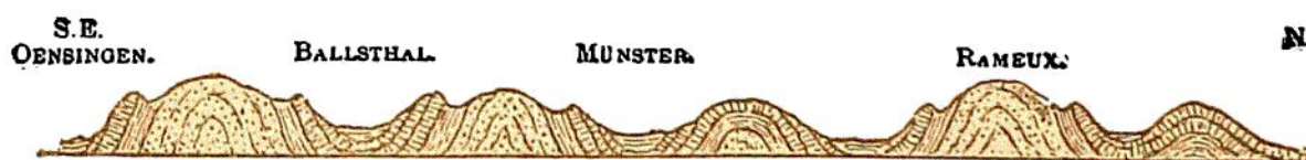
Fig. 464.—Symmetrical Flexures of Swiss Jura (the ridges coinciding with anticlines and the valleys with synclines).
