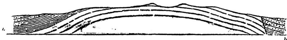
Fig. 465.— Uinta Type of Flexure. a, Palæozoic rocks; b, Mesozoic; c, Tertiary; f, fault.
