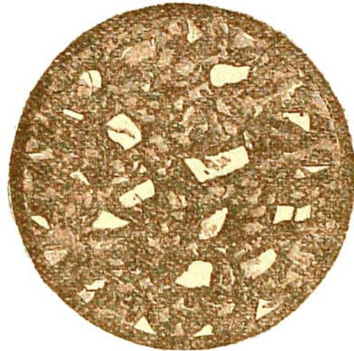
Fig. 22.—Clastic Structure, of Organic Origin—Structure of Chalk (Sorby). Magnified 100 Diameters. (See p. 246.)
