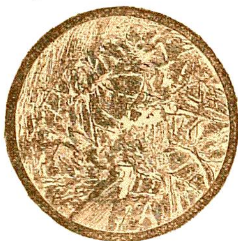
Fig. 34.—Microscopic Structure of Serpentine (20 Diameters).
