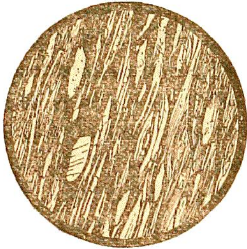
Fig. 80.—Section of compressed argillaceous rock in which cleavage structure has been developed. Magnified. (Compare Fig. 256.)
