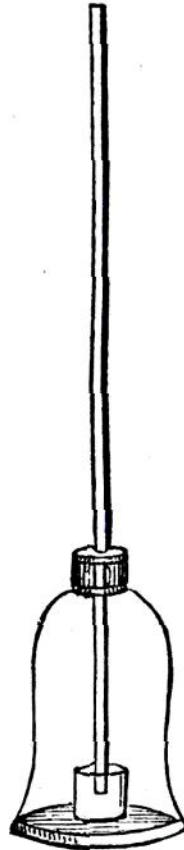
Experiment showing the influence of the atmosphere on the mercurial column.
