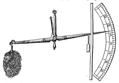
and a slender rod or index at the other. The sponge, which may be rendered more hygrometric if steeped in pearlash and water, rapidly absorbs moisture from the air; and as its weight increases the index rises, and gives a proportional estimate of the vapour which may be present in the atmosphere.
