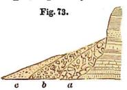
Fig. 73 represents a cliff, at the base of which there is produced a talus of large angular blocks, a. These are further acted upon at b, and c, until the rains or tides remove the finer portions in the form of mud.
