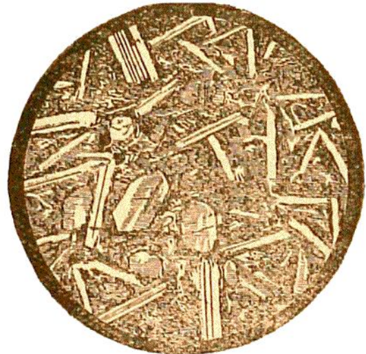
Fig. 16. —Hemi-crystalline Structure. Dolerite, consisting of a triclinic Felspar, Augite, and Magnetite in a devitrified Ground-mass (20 Diameters). The numerous narrow prisms are triclinic Felspar; the broader monoclinic forms, slightly shaded in the drawing, are Augite; the black specks are Magnetite; the needle-shaped forms are Apatite. (See p. 294.)
