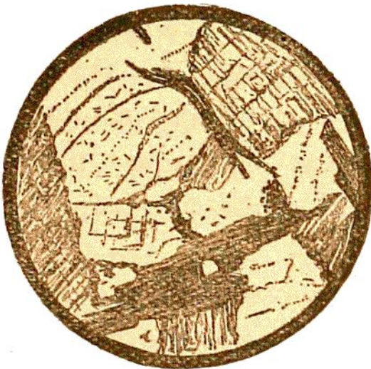
Fig. 15. —Holocrystalline Structure. Granite (20 Diameters). The white portions are Quartz, the striped parts Felspar, the long, dark, finely striated stripes are Mica. (See p. 273.)
