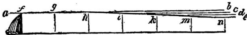
Fig. 120.—Section to illustrate the lowering of Lake Erie by the recession of Niagara Falls.
