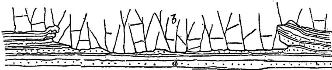
Fig. 285.—Section at base of south front of Salisbury Crags, showing portion of strata cut out by intrusive diabase. a , sandstones, shales, etc.; b , diabase. Length of section, 22 feet.
