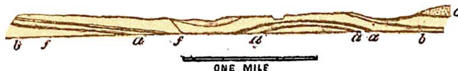
Fig. 304.—Section of intercalated diabase (toadstone) in Carboniferous Limestone, Derbyshire (B.). a a , Toadstone, in two beds; b b , Limestones; c , Millstone grit; f f , Faults.
