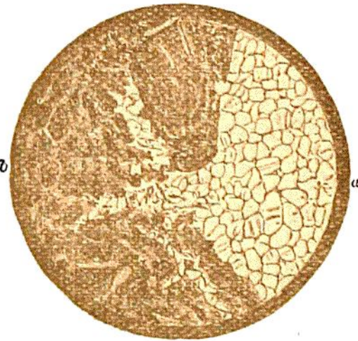
Fig. 310.—Section of limestone (a) (Burdie House) converted into granular marble by basalt (b). Magnified 20 diameters.
